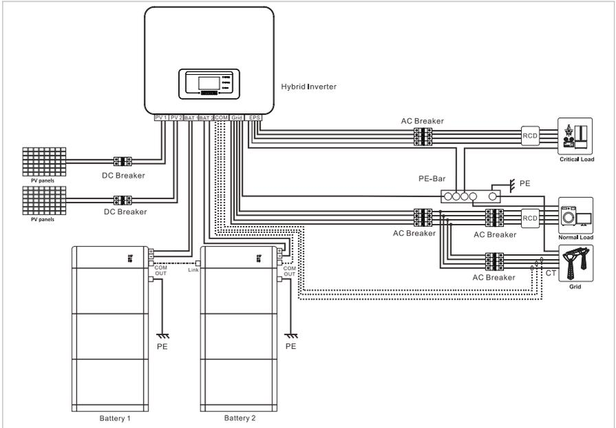
Below is the schematic connection diagram of a system where the neutral line and ground line are connected together.
