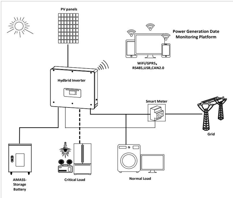
HYD 5K...20KTL-3PH inverters may only be used with photovoltaic modules which do not require one of the poles to be earthed. In
