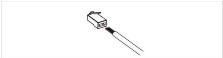
2. Route the cable terminal through the cable gland and insert the communication cable into the RJ45 connector.
