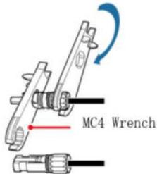
7. Insert the positive and negative connectors into the corresponding DC input terminals of the inverter until you hear a “clicking” sound.
