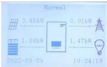
If PV generation is larger than the load consumption, the surplus power is stored in the battery
