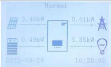
If the PV generation is less than the load consumption, it will discharge the battery to supply power to the load.
