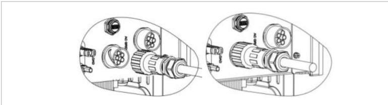
5. Connect the AC connector to the AC connection of the inverter by turning it clockwise until it locks into place.
