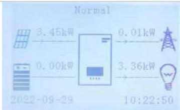
If PV generation equals the load consumption ( $\Delta P < 100 \text{ W}$ ), the inverter won't charge or discharge the battery
