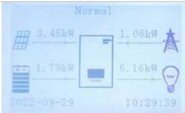
If PV generation plus Battery discharge power is less than the load, the inverter will import power from the grid.
