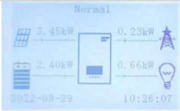
If the battery is full or at maximum charging power, the excess power will be exported to the grid
