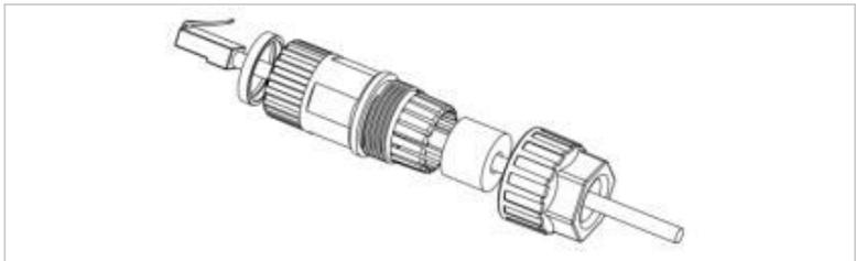
3. Lock the connector by turning clockwise:
