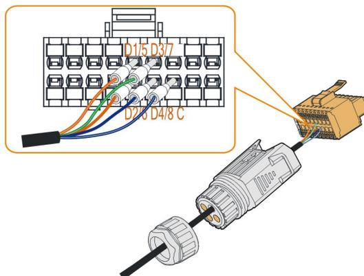
figure 5-10 Connexion DI
