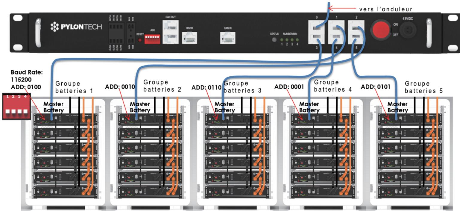
*Each battery pile can configue maximum 8pcs US2000B Plus or 8 pcs US3000*
